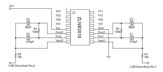
The following circuit shows the additional components that will be used for polarisation mode and 22kHz tone detection in typical ZLNB2006/9 application
